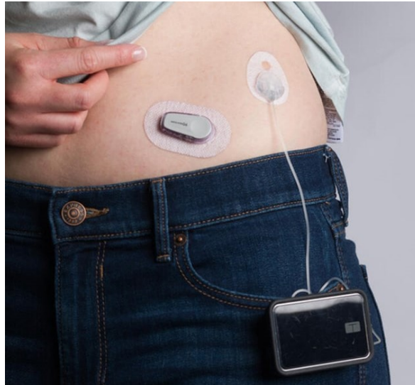
Figure 1: Continuous insulin administration system with an insulin pump and a CGM device [14].
